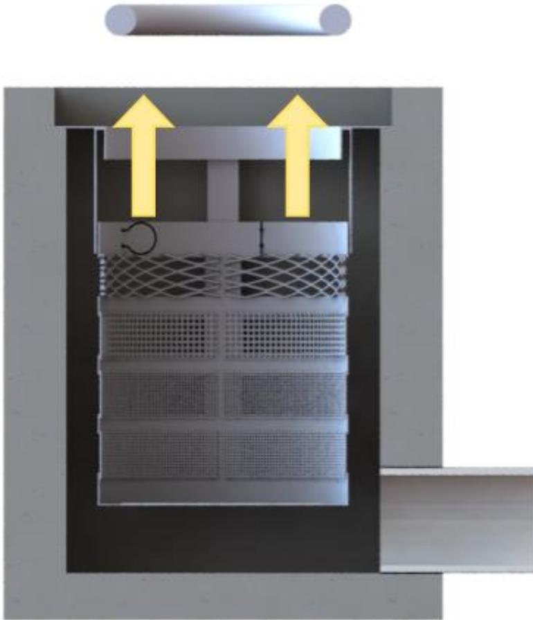
Remove the hydrocarbon boom that is attached to the inside of the filter basket. The hydrocarbon boom is zip tied to the top perimeter of the filter. Assess the color and condition of the boom using the following information in the next bullet point. If replacement is required, install and fasten on a new hydrocarbon boom.
