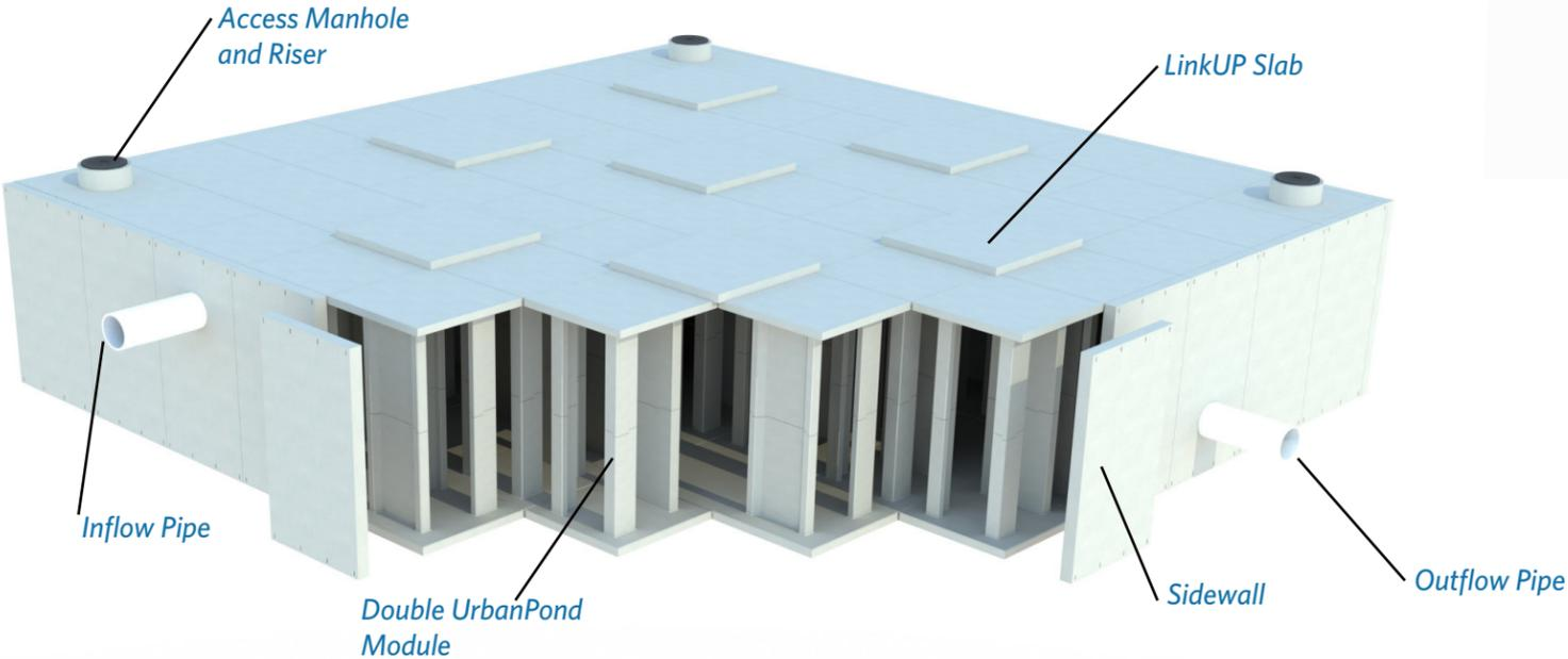
LinkUP Slabs span the open cavities in a 9-module array.
