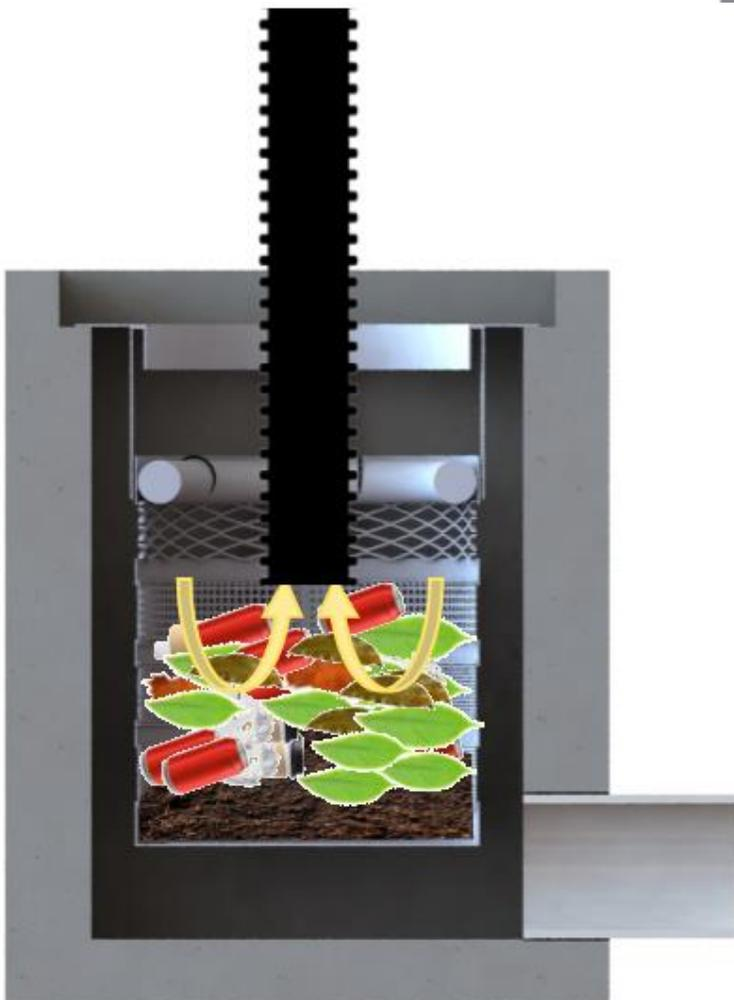
Insert the vacuum hose down into the filter basket and suck out debris. Use a pressure washer to assist in vacuum removal. Pressure wash off screens.
